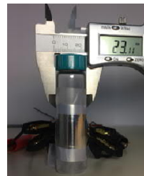
Fig 2. Supercapacitor statically bent to 2.3 cm cylinder and measured.
