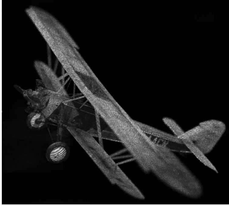
Figure 5. Numerical small aperture reconstruction of one viewpoint from a 64k \times 64k hologram computer-generated from the JPEG PlenoDB bi-plane point cloud with the 10 million points.
