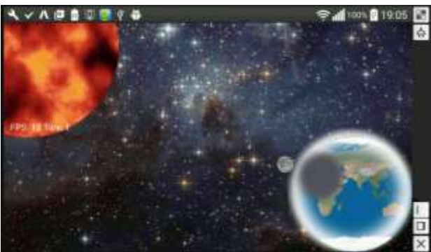
Figure 3. The test application (captured from mobile browser) and its animated objects: Sun (upper left corner with animated lava texture), Earth (lower right corner, rotating), Moon (small grey circle close to earth), Moon shadow (larger half-transparent grey circle on Earth surface), Earth atmosphere (light half-transparent halo surrounding Earth).
