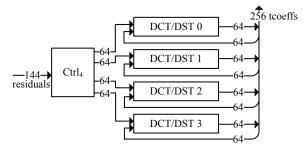
Figure 3. Block diagram of the 4-point DCT/DST unit.
