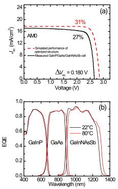
Figure 1. (a) AM0 biased IV-characteristics of GaInP/GaAs/GaInNAsSb solar cell and the simulated performance of GaInP/GaAs/GaInNAsSb cell. (b) EQE characteristics of GaInP/GaAs/GaInNAsSb solar cell measured at 22°C and 80°C.
