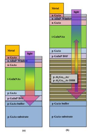
Fig 1. Generic test structures for the GaInNAs solar cells with AlInP window and GaInP back surface field (BSF) layers: (a) single junction GaInNAs solar cell and (b) GaInNAs solar cell with a DBR back reflector.
