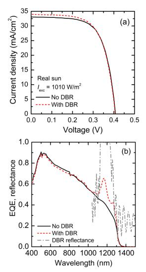
Fig. 2. (a) Measured LIVs from GaInNAs solar cells with and without DBR reflectors. (b) EQE and reflectance values for GaInNAs solar cells with and without DBR reflector showing the improvement of photocurrent in the GaInNAs junction.
