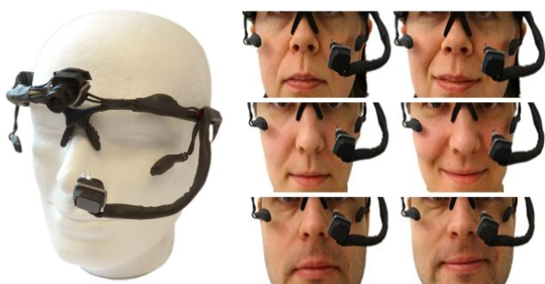
Figure 1: Left: Wearable prototype for pointing by gaze and selecting by smiling. Right: Examples of smiling movements (from neutral to smile) for producing a click by smiling.
