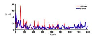
Fig.6. Errors of Kalman filtered position estimate versus the error given by the BRAIM method on a real GPS data vehicular test.
