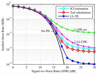
Fig. 6. Simulated SER as a function of SNR. PN is generated with PLL-based oscillator. AWGN channel is used.
