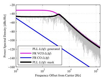
Fig. 1. Example of PLL output phase noise for centre frequency of 1.5915 GHz.
