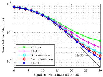
Fig. 5. Simulated SER as a function of SNR. PN is generated with freerunning oscillator ( $\beta$ =200 Hz). Extended ITU-R Vehicular A channel model is used.
