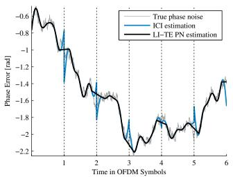
Fig. 3. LI-TE method demonstrated for a free-running oscillator with 100 Hz spectral width ( $\beta$ ) over six OFDM symbols. For demonstration purposes, only one iteration in ICI estimation is used.
