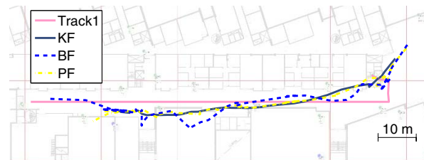
Figure 4: KF, BF and PF estimates for test track 1
