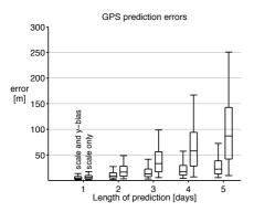
Fig. 3. Prediction errors for GPS satellites with the different solar radiation pressure models.
