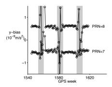
Fig. 2. Time series of y-bias acceleration  $\alpha_2$  estimates for GPS satellites PRN 7 and PRN 8. Shaded areas represent eclipse seasons.
