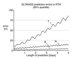
Fig. 6. 95%-quantile of the prediction errors in the RTN reference frame for GLONASS satellites.
