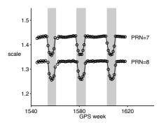
Fig. 1. Time series of scale parameter  $\alpha_1$  estimates for GPS satellites PRN 7 and PRN 8. Shaded areas represent eclipse seasons.
