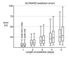
Fig. 4. Prediction errors for GLONASS satellites with the different solar radiation pressure models.
