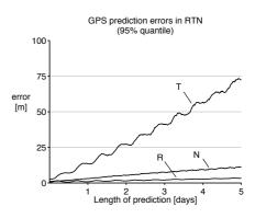
Fig. 5. 95%-quantile of the prediction errors in the RTN reference frame for GPS satellites.
