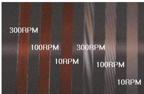
Fig. 8 UV curing film of micro structures with different spindle speed
