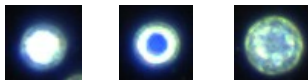
Figure 5.5: Different reflection of different materials. Left to right: aluminum, polystyrene and glass.
