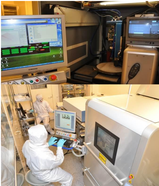
Figure 10. Picosecond laser setup change to a femtosecond laser setup at the workstation.
