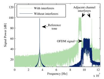
Fig. 2. Example spectra of the reference tone, the OFDM signal and the interferers after aliasing by sub-sampling at 245.76 MHz with 20 ps RMS jitter. The original RF signal centre-frequency is 2.6 GHz while the reference tone frequency is 36 MHz.
