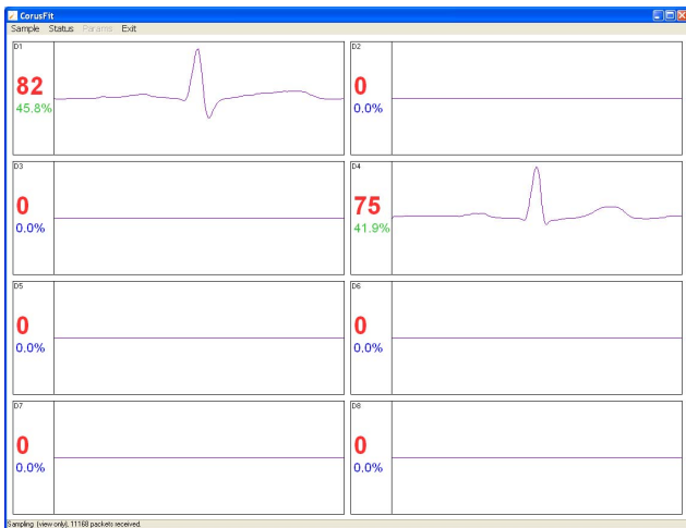
Fig. 2. User interface of the PC software. Current heart rate value, percentage from the maximum heart rate, and an average QRS-complex are shown for each trainee.
