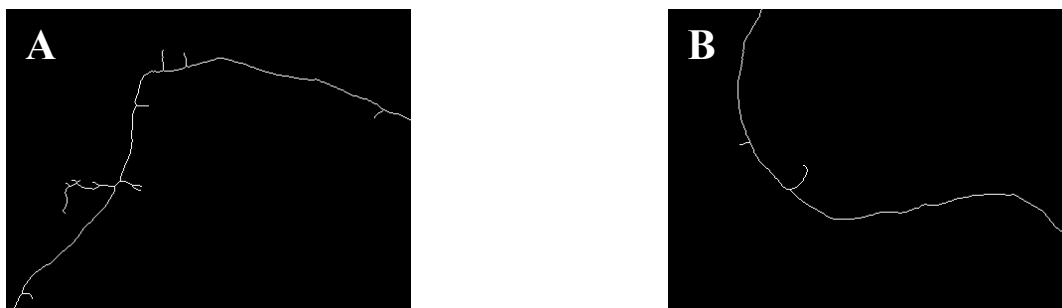
Figure 4. Close-ups of Fiber 1 (A) and Fiber 2 (B) after morphological thinning of the image.
