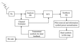
Fig. 2. Receiver model with IF.
