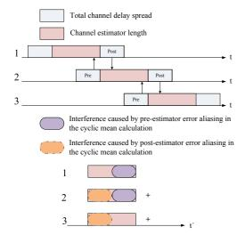
Fig. 4. Illustration of the error aliasing phenomenon when using short channel estimator. Here three copies of the cyclic pilot sequence are drawn, which have shorter length than the channel delay spread. The lower part of the figure models the summation in the cyclic mean calculation.
