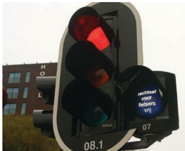
Figure 117. Right turn on red for cyclists indicated on a signal support. (Delft)
