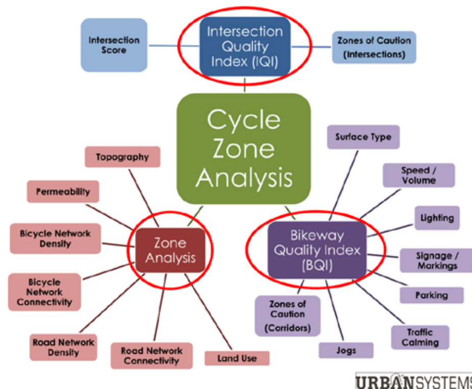
Fig. 12. The Cycle Zone Analysis evaluates cycling potential based on three different sectors. (Figure: Fadum & Patterson, 2010)
