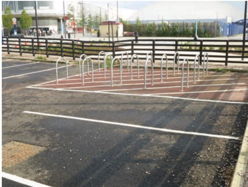
Figure 144. Parking bays converted for bicycle parking (London).
