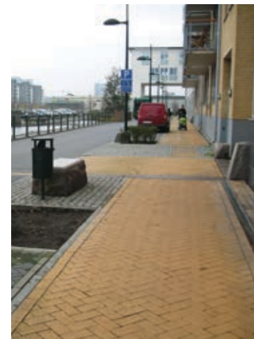
Fig. 22. In a Malmö residential area, the pathways are clearly indicated in a specific yellow colour. The street furniture is located to the side of the path so as not to obstruct the traffic.
