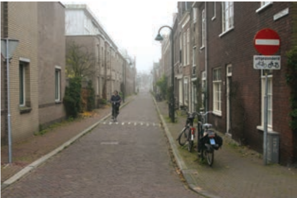
Figure 83. The narrow streets of this Delft residential area accommodate mixed traffic. To facilitate cycling, cyclists are permitted to cycle against the one-way traffic.
