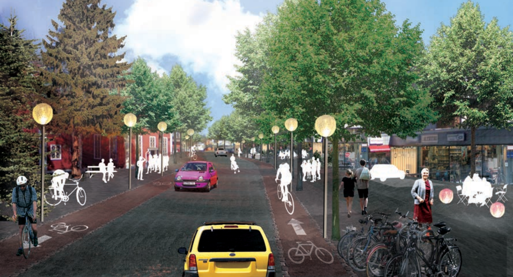
Figure 49. By making the street narrower and restricting the on-street parking, it would be possible to have one-way cycleways on Uudenmaankatu in Hyvinkää.
