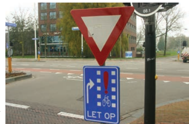
Figure 118. A sign warning the motorist turning right of the cyclists going straight on. (Delft)
