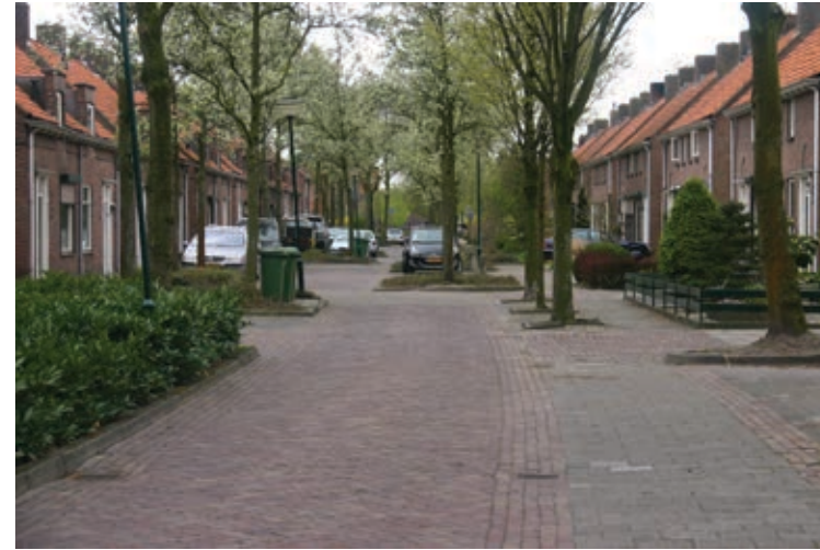
Figure 89. In the Netherlands, horizontal deflections are used to slow down driving speeds on the access roads. (Rijen)
