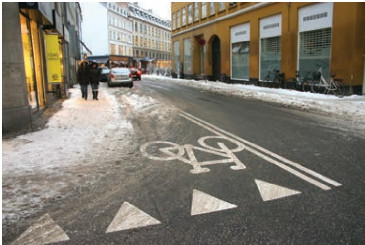
Figure 96. Street markings for the cyclists riding against the traffic in a Copenhagen intersection.
