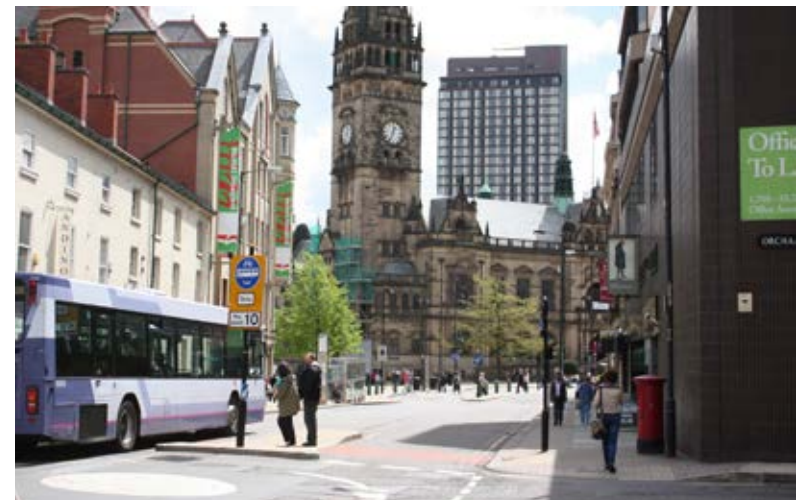
Fig. 40. Public transport street crossing located between two pedestrian areas in Lund (above). The same high-quality pavement outside the pedestrian area creates an image of extension to the area. Sheffield's Leopold Street, for public transport (below), is of the shared space type, with no barrier effect to pedestrians.
