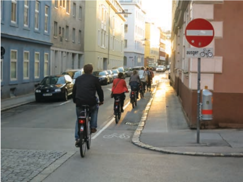
Figure 94. Cycling against the traffic on a one-way street with a cycle lane. (Vienna)
