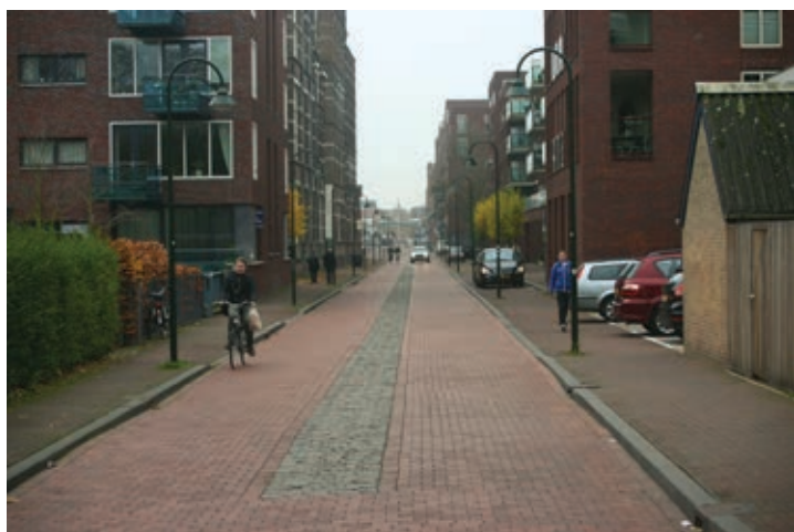
Figure 75. This street running through a residential area was converted into a bicycle boulevard. (Delft)
