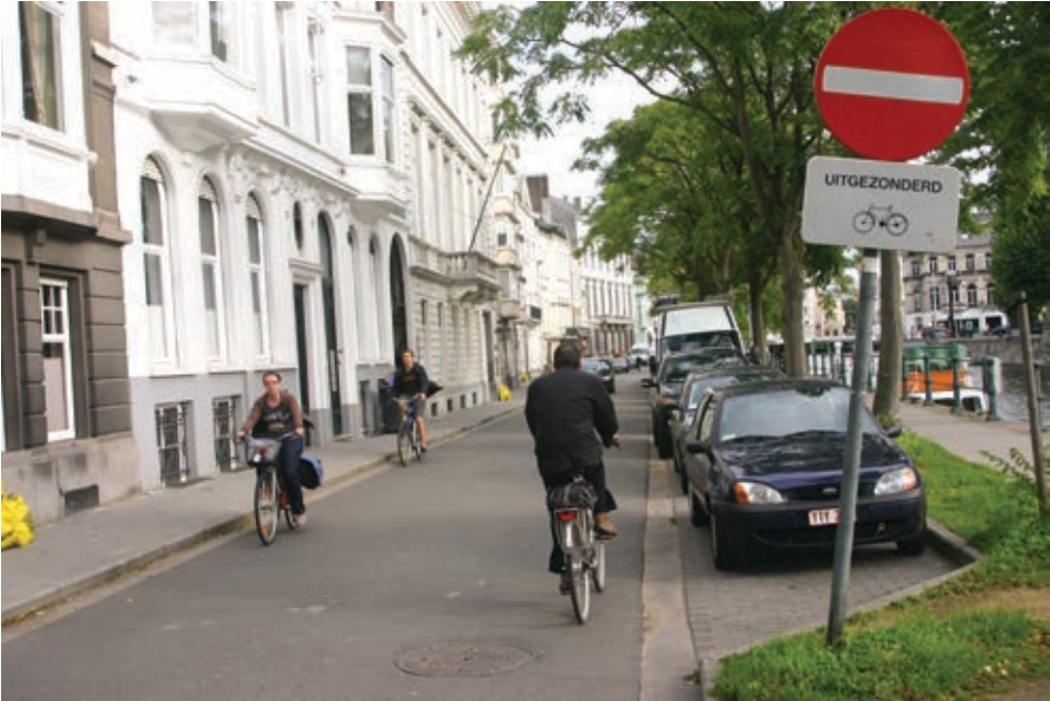
Figure 93. It is advisable to permit cycling against the traffic on one-way streets. It makes cycling faster and easier by eliminating unnecessary detours. (Ghent)
