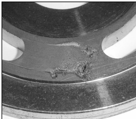
Figure 2. Valve plate with cavitation wear due to bad operation conditions.
