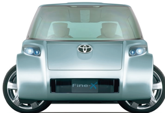
Figure 7: Toyota Fine-X concept car having 4 in-wheel electric hub motors
