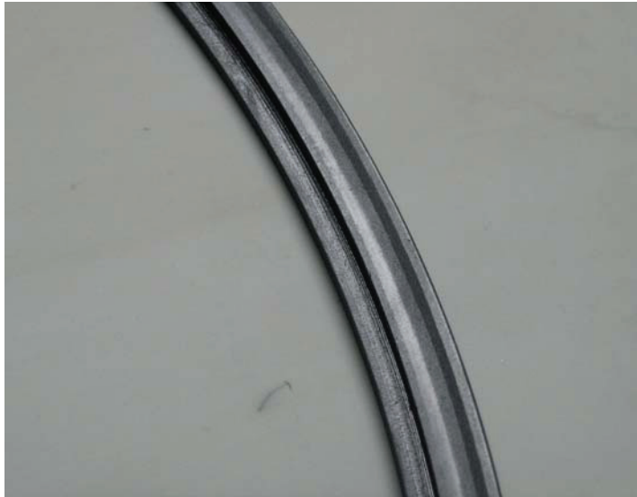
Figure 10. Seal A after tests. Attachment flange to the left and seal lip to the right.
