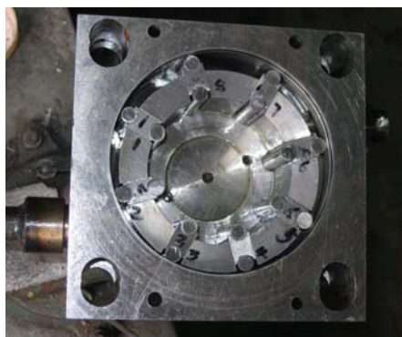
Fig. 23 The structure drawing of the same width, double-action, four-output pump and motor with double-stators and connecting rods
