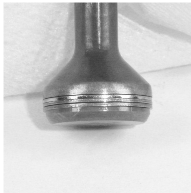
Figure 7. Piston after 3.9 million cycles.
