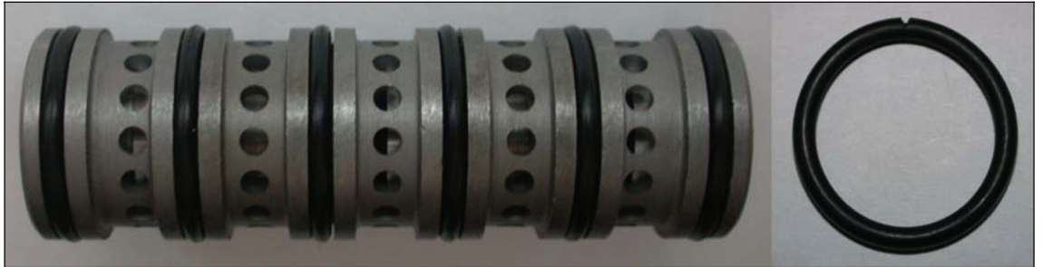
Fig. 3: Spool sleeve of the valve and a seal crack.
