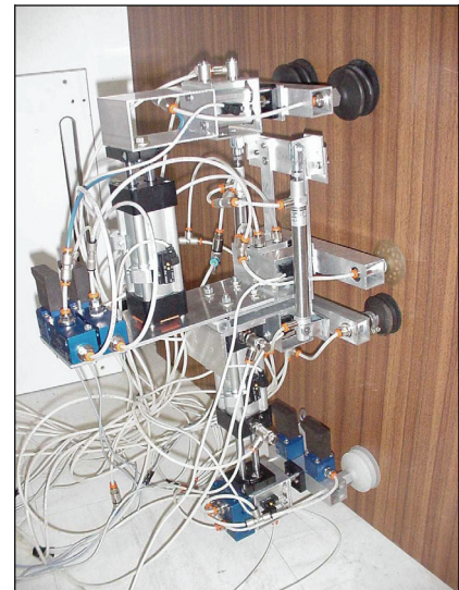
Fig. 10: Motion phases: a) motion on horizontal plane; b) approaching to vertical plane; c) intermediate climbing phase; d) motion on vertical plane.
