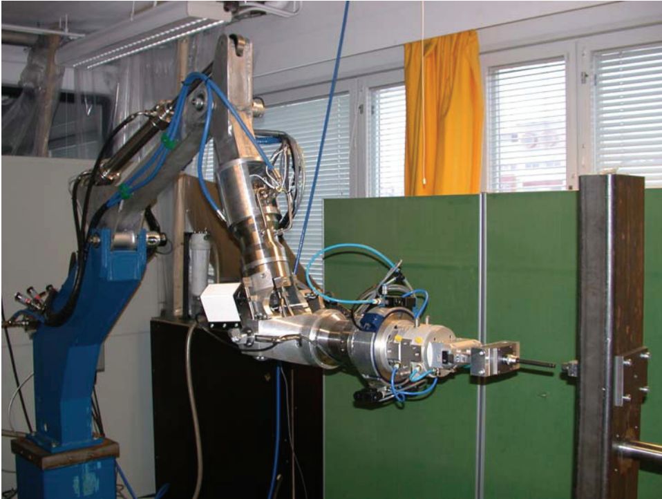
Figure 3: 5 DOF WHMAN with a wrench tool
