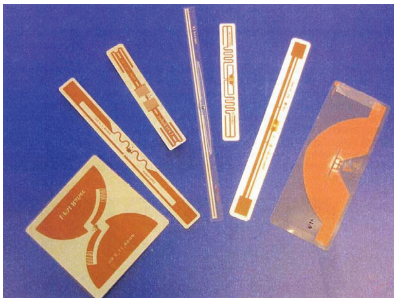
Figure 2. Different dipole-type UHF tags [7]
