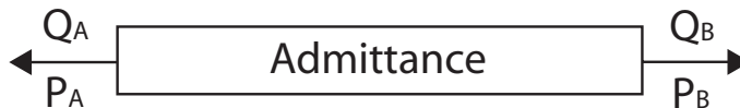
Figure 6: Flow and pressure in equation (10) are correlated with each other through an admittance.
