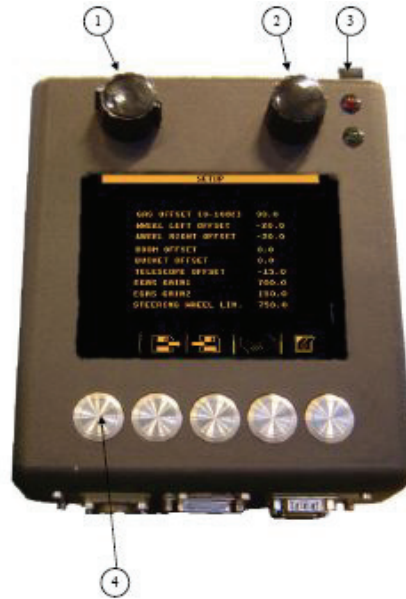
Figure 4: Control and display module. (1) A screen handle selector (2) Change value handle (3) Main power switch (4) Selection buttons
