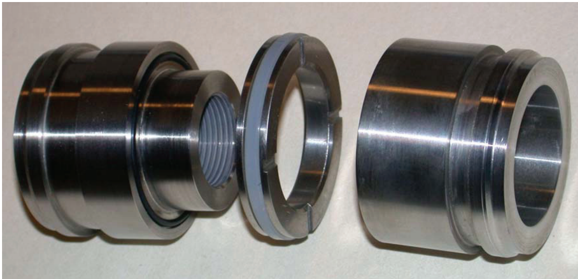
Figure 4. Seal carrier in the middle of two part piston.
