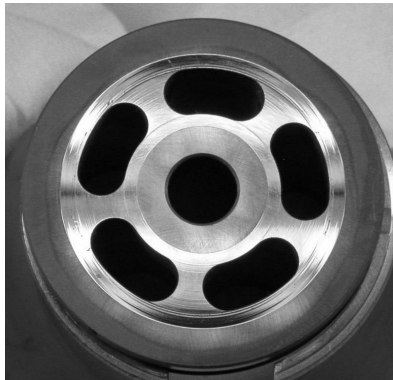
Figure 8. Cylinder barrel after 3.9 million cycles.
