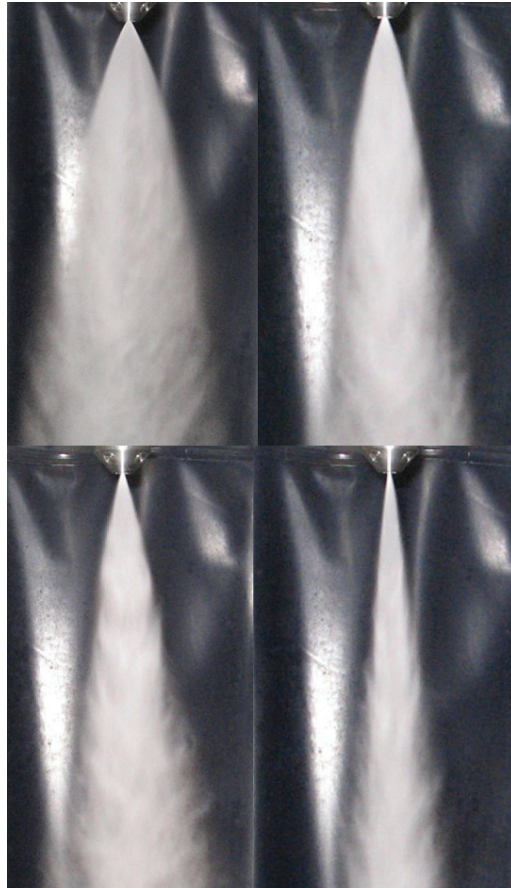
Picture 13. Same nozzle with different end boring sizes
