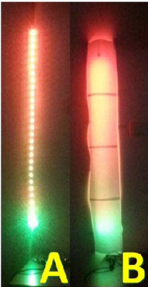
Figure 5: Displaying the image without (A) and with the installed paper diffuser (B)
