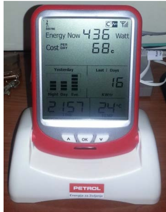
Figure 1: CurrentCost electrical energy meter control unit
