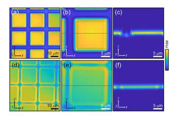
**Fig. 3.** Transversal *xy* THG microscopy images of the (a,b) developed and (d,e) undeveloped photopolymerized structures in a SU-8 film on silicon wafer. Longitudinal *xz* THG microscopy images of the (c) developed and (f) undeveloped samples. The locations of the longitudinal planes are marked in (b,e). Image resolution is 100 pixels  $\times$  100 pixels.
