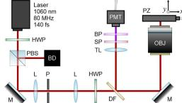
**Fig. 1.** Schematic diagram of THG microscopy setup. The microscope is powered by a laser source (1060 nm, 80 MHz, 140 fs,) and composed of the following components: half-wave plate (HWP), polarizing beamsplitter (PBS), beam dump (BD), lenses (L), mirrors (M), pinhole (P), dichroic filter (DF), microscope objective (OBJ), piezo-scanners (PZ), tube lens (TL), shortpass filter (SP), bandpass filter (BP) and photomultiplier tube (PMT).
