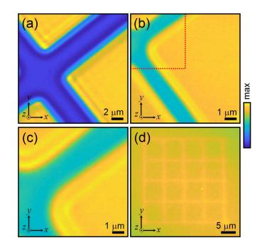
**Fig. 4.** High-resolution transversal *xy* THG microscopy images of the (a) developed and (b,c) undeveloped photopolymerized structures in a SU-8 film on silicon wafer. The THG image in (c) is marked in (b). (d) Transversal *xy* THG microscopy image of a three-photon polymerized microstructure in a thick SU-8 film on silicon wafer. Image resolution is 100 pixels  $\times$  100 pixels.
