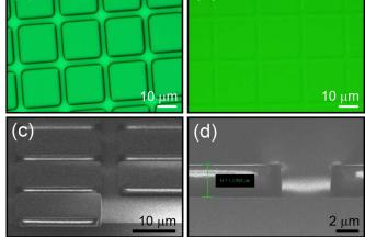
**Fig. 2.** Bright-field optical microscopy images of the (a) developed and (b) undeveloped photopolymerized structures in a SU-8 film on silicon wafer. (c) Oblique and (d) side-view SEM pictures of the developed film.
