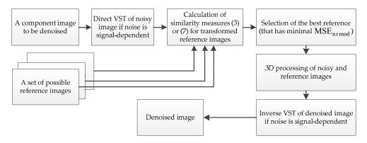
**Figure 3.** Block-diagram of the proposed processing approach. VST—variance stabilizing transform; MSE—mean square error.
