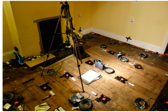
Figure 4. Instrumentation set-up on the bare floorboard surface of the case-study house.
