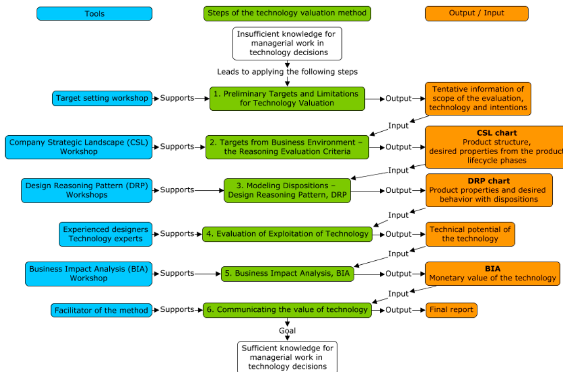
Figure 4. A description of the proposed technology valuation method (TVM), with the knowledge-gathering tools that are used and the outputs that document this knowledge.
