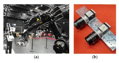
**Figure 2.** An example of the setup for acquiring the datasets; (**a**) robotic arm moving in the workspace; (**b**) cameras and Lenses for data acquisition.
