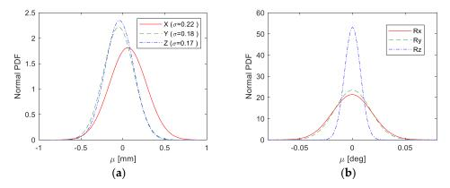
**Figure 6.** Probability distributions functions; (**a**) the measured position error from the robotic arm; (**b**) the modeled orientation error for the robotic arm.
