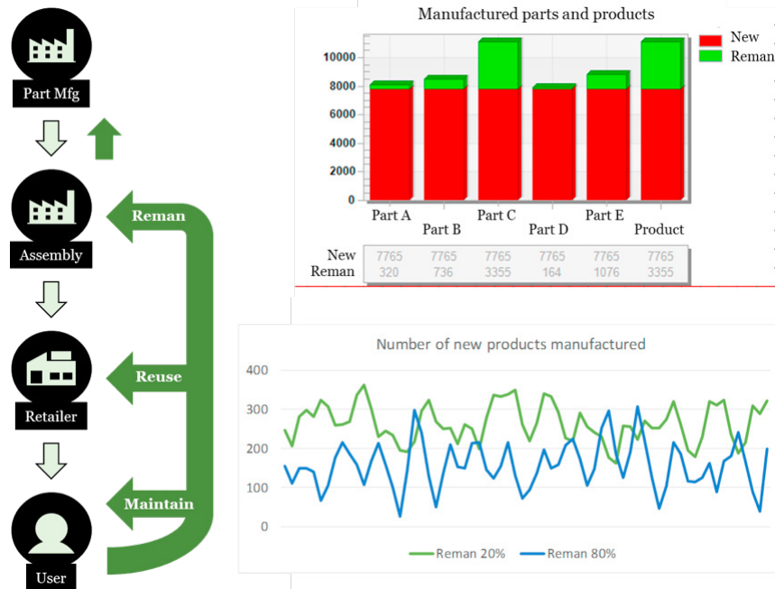
Fig. 2. The principle of the closed-loop material flow simulation exercise and example results.
