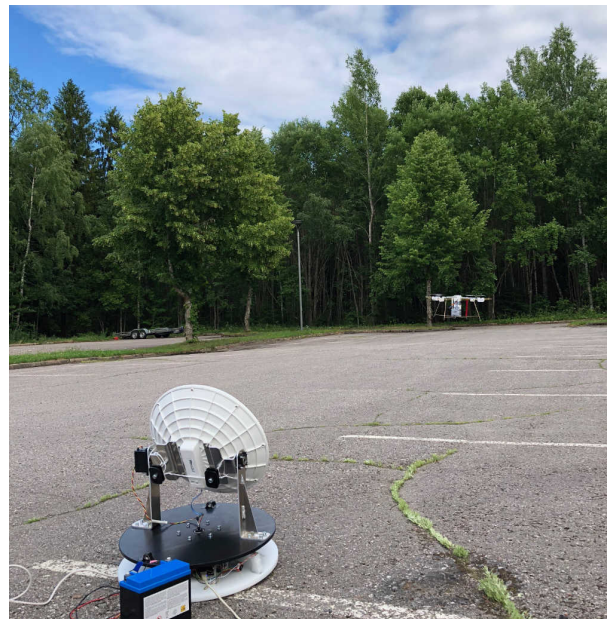
Fig. 9. Equipment for propagation measurements.
