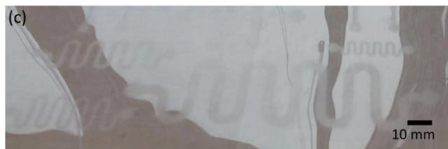
Figure 2. a) Computer-aided drafting (CAD) design of surface patterns for droplet control tests. Photos of b) laser-cut stencil mask and c) spray-coated CNF patterns on PET substrate.
