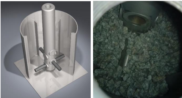
Figure 1: High speed slurry-pot on the left as 3D illustration and on the right the same device with dry-pot test method showing a test sample inside the abrasive bed before completing the abrasive filling.
