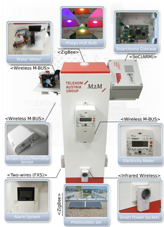
Fig. 4: Key hardware components of SyMPHOnY platform. may be infeasible to offer the universal home gateway as a "one-box" solution (mindful of target price for the "complete package").
