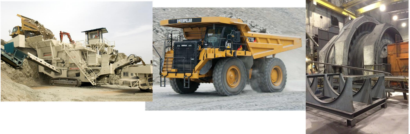
Figure 4.2.1 Three case studies were carried out for detailed energy and cost analysis: a mobile jaw crusher, an off-highway haul truck and a grinding mill.
