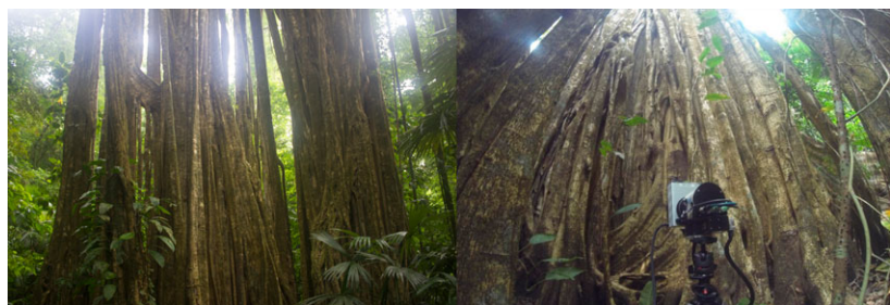
Figure 6. Photographs of the exterior (left) and interior with CBL1 (right) of the strangler fig (Costa Rica). The geometric complexity of the many separate stems created challenging patterns of occlusion that could only be mitigated by leveraging the compactness and rapid scanning of the CBL. CBL, compact biomass lidar.
