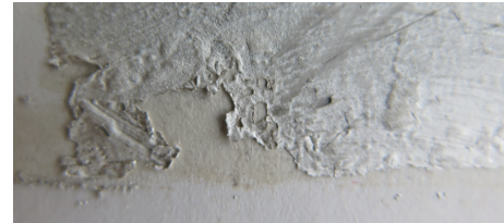
FIGURE 7: A close-up photo of burned antenna in Sample 13.
