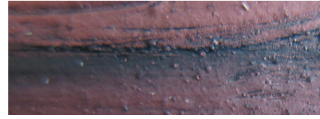
FIGURE 6: A close-up photo of partially sintered antenna in Sample 7.
