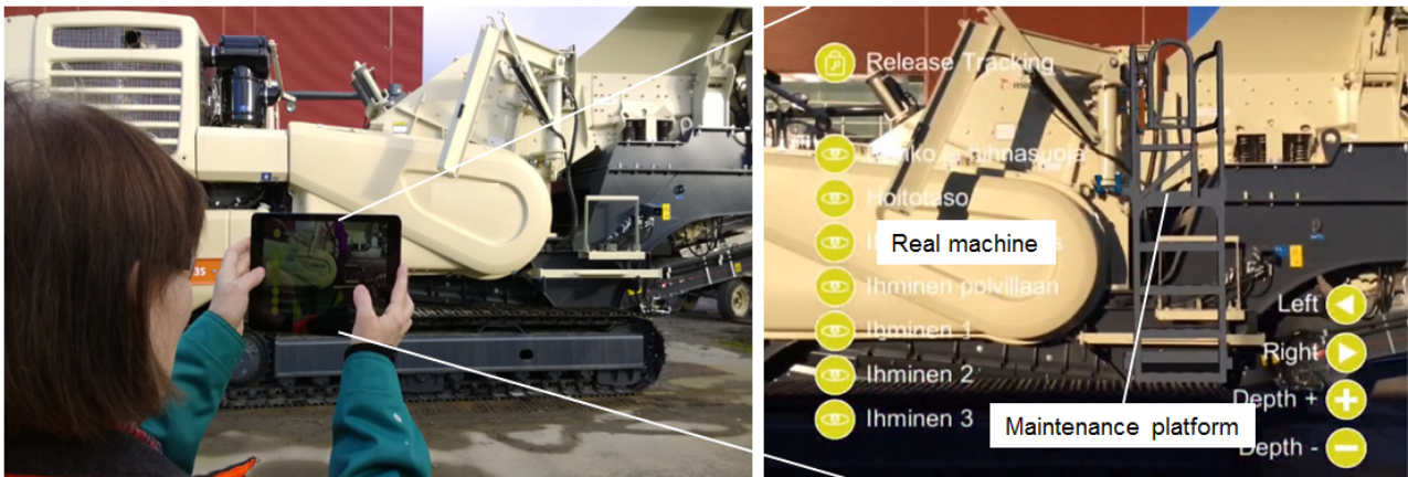
Figure 1. The augmented reality system for reviewing the maintenance platform. A participant is holding a tablet PC in her hand on the left-hand side. On the right-hand side is a screenshot from the tablet PC: a 3D model of a maintenance platform is augmented on top of the real machine.
