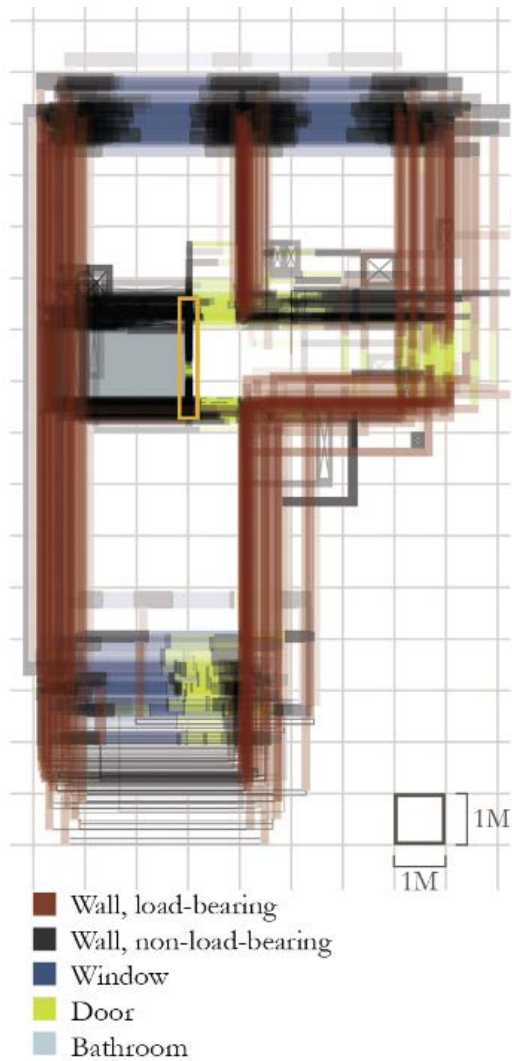
FIGURE 2 The method for creating the flat types in Kaasalainen and Huuhka (2015a) and the variation in the dimensions of the flats, scale 1:250. As the figure illustrates, the type plans (Figure 3) were the result of piling translucent line-weighted color-coded graphs that were made from the original plan drawings, aligned along the circled bathroom front wall, and by defining mean values for the dimensions of rooms and locations of windows and doors visually. (Kaasalainen & Huuhka, 2015a).
