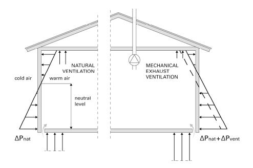
Pressure differences created by the stack effect  $\Delta P_{nat}$  and forced exhaust ventilation  $\Delta P_{vent}$ . The arrows describe the pressure difference and direction of air flow. The curved arrows indicate the flow of radonbearing soil air. 185x121mm (300 x 300 DPI)
