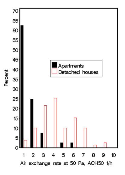
Distribution of the ACH<sub>50</sub> leakage factor in newly built wooden-frame detached houses (1995–2005, n = 79) and apartments with concrete structures (2001–2003, n = 40)<sup>(7, 8)</sup>. The upper limit of the ACH<sub>50</sub> categories is presented. 200x226mm (72 x 72 DPI)
