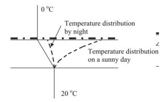
**Figure 3.** Rough summary of the typical diurnal thermal performance of an AAC roof structure (Lindberg et al., 2008).
