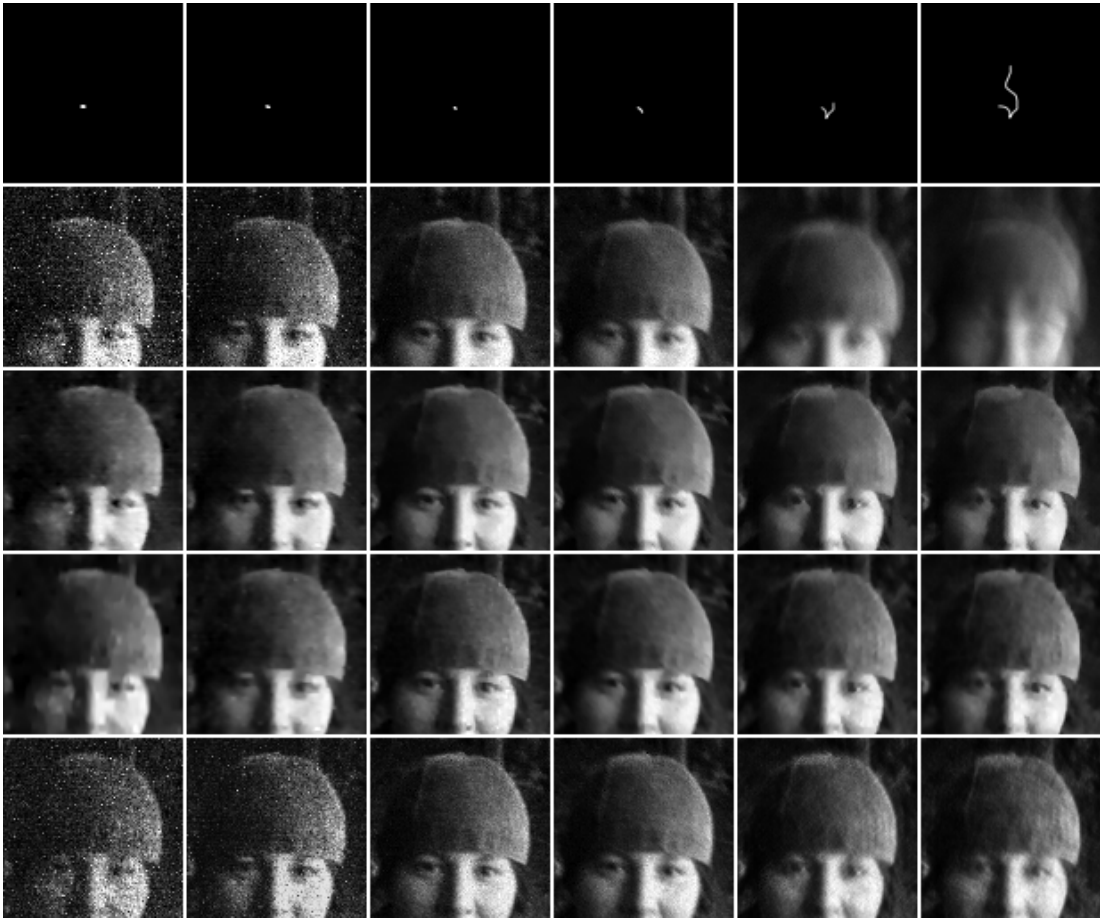
Fig. 11. An example of raw data acquired from Liza (green channel). The top row contains the estimated PSFs: the blur develops along trajectory e ). The second row contains the camera raw data, acquired with settings (from left to right): 2, 3, 5, 6, 8, 10. The remaining rows show the restored images using different deconvolution algorithms. Third row: Anisotropic LPA-ICI Deconvolution, RMSE values (from left to right): 10.01, 7.56, 5.19, 5.61, 6.09, 8.99. Fourth row: Deconvolution using Natural Image Priors, RMSE values (from left to right): 9.79, 7.57, 5.18, 5.16, 5.54, 8.16. Bottom row: Richardson-Lucy Deconvolution, RMSE values (from left to right): 28.43, 18.25, 8.47, 7.33, 7.12, 9.43. Image intensities have been rescaled for visualization purposes.
