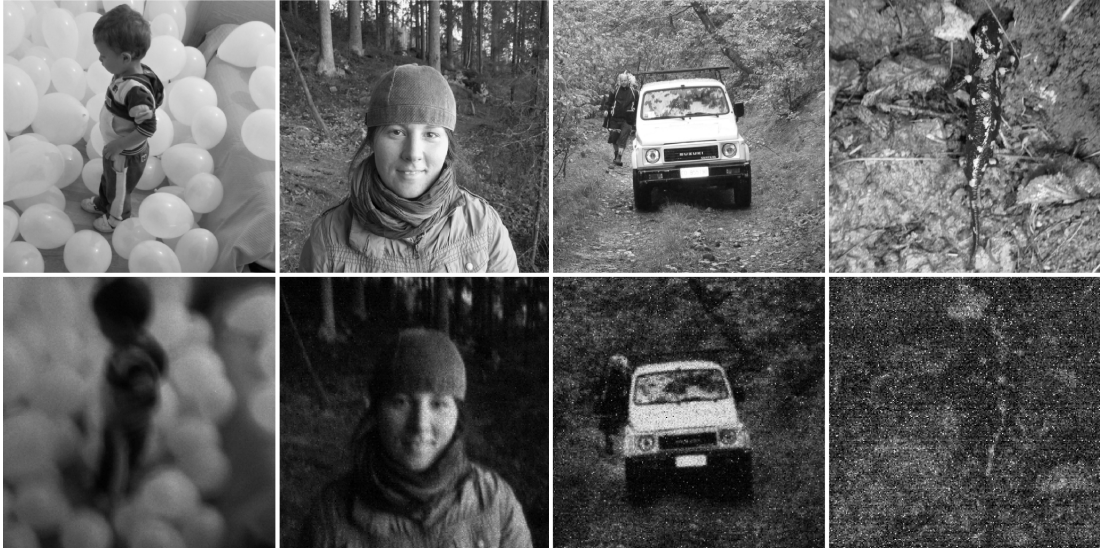
Fig. 8. Top row: the natural images ( Balloons , Liza , Jeep and Salamander ) that were used to render the movies for the experiments. Bottom row: examples of the captured raw images demonstrating that there is a clear blur/noise trade-off; these four images have been acquired with settings 10, 8, 6, 4, 2 (see Table I), and come from the trajectory f), d), b), e) and a), respectively. Images were taken from the blue channel and rescaled for visualization purposes.
