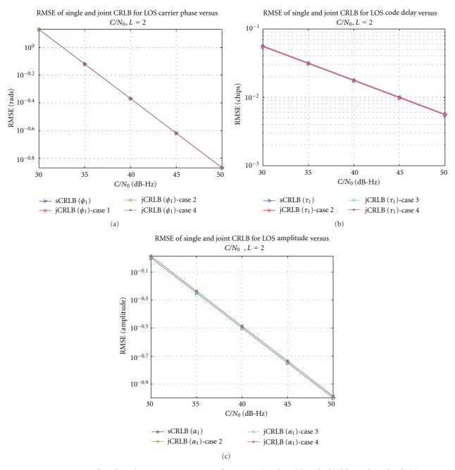
FIGURE 3: RMSE of Single and Joint CRLB versus  $C/N_0$  for LOS carrier phase (a), code (b) delay and amplitude (c).
