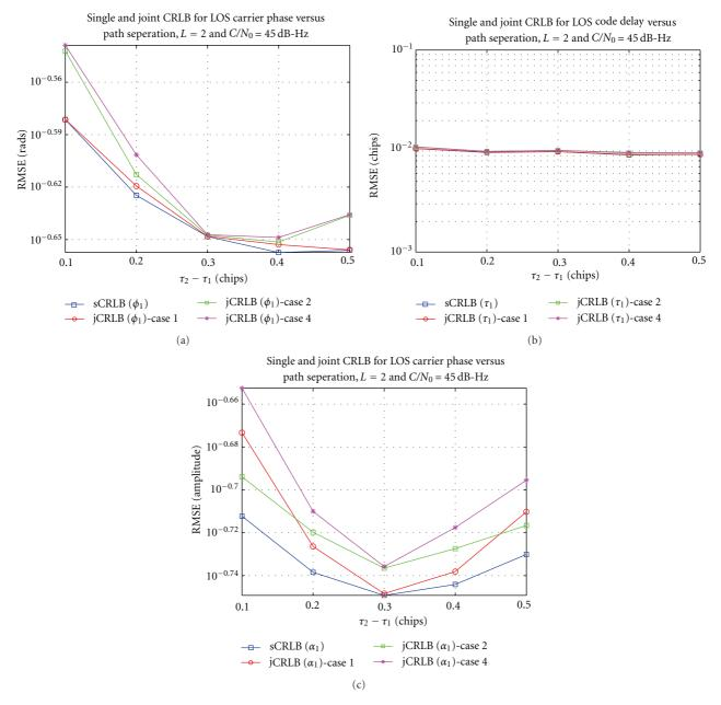
FIGURE 2: RMSE of single and joint CRLB versus path separation ( $\tau_2 - \tau_1$ ) for LOS carrier phase (a), code (b) delay and amplitude (c), L = 2 and  $C/N_0 = 45$  dB-Hz.
