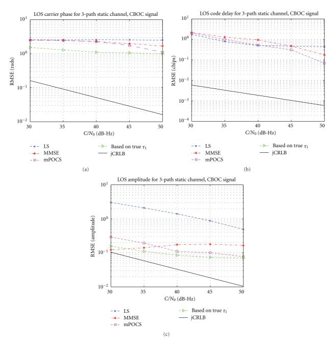
FIGURE 6: LOS carrier phase (a), code delay (b), and amplitude (c) versus  $C/N_0$  for 3-path static channel and CBOC signal.
