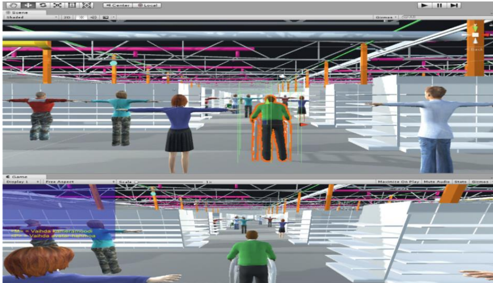
Fig. 3. A simulation application realized with the Unity game engine. A game collider corresponding to the spatial need of an avatar is visible on the picture.
