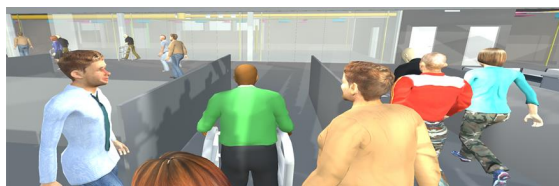
Fig 5. The simulation is active and smoke begins to enter the interior of the supermarket. The profiled customers (game objects) are rushing in chaos towards the defined emergency exits under the control of the AI engine (the reaction phase and the mobilization phase).
