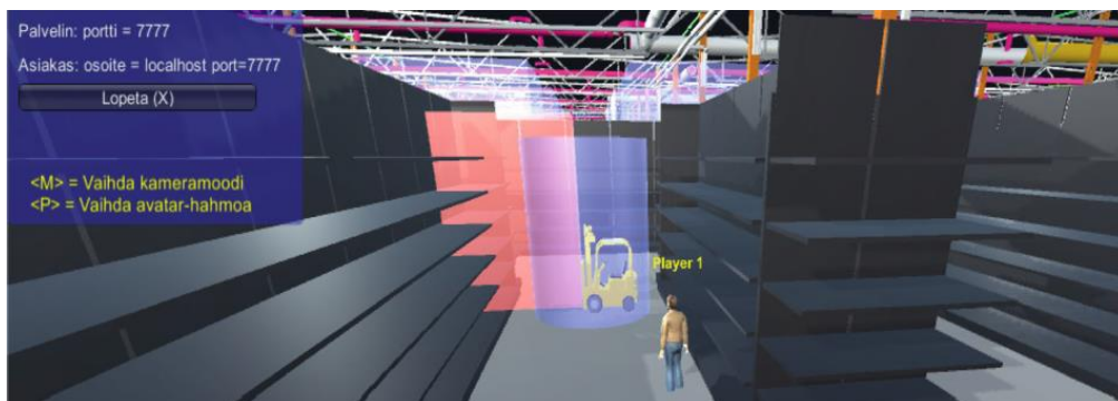
Fig. 12. A forklift with added game colliders and the added reachability region operates in a warehouse and the player of the piloting application exists in the same space.
