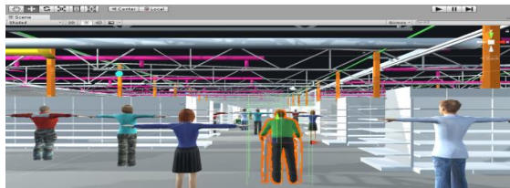
Fig 4. A simulation application realized with the Unity game engine. A game collider corresponding to the spatial need of an avatar is visible on the picture.
