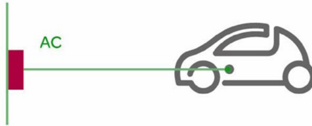
Figure 3. EV charging mode 1 [26]
