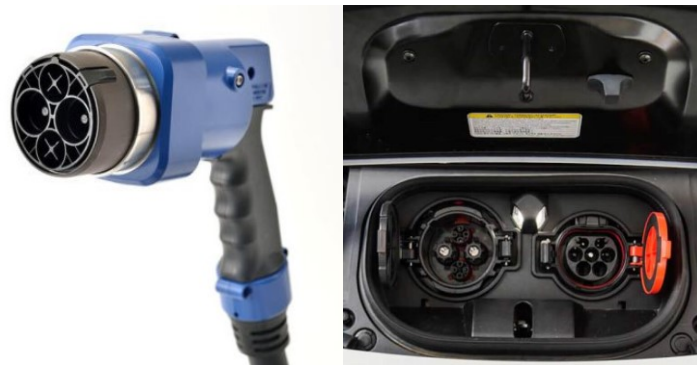
Figure 8. CHAdeMO connector (left) and two socket combination with CHAdeMO and Type 2 connectors (right) [36]
