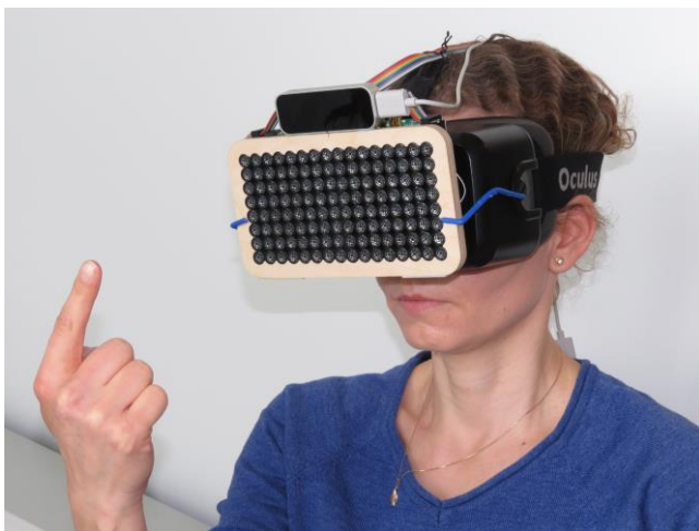
Figure 4: Mid-air tactile feedback can focus ultrasound waves to user's finger or palm, which are here tracked with Leap Motion. The system can be used with any HMD, here with Oculus Rift.
