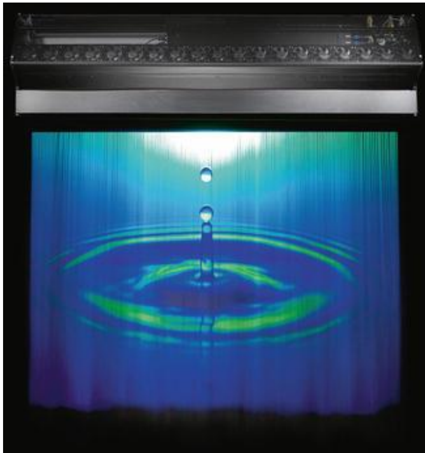
Figure 2. A large fogscreen hanging from the ceiling showing a projected image on a thin layer of fog.
