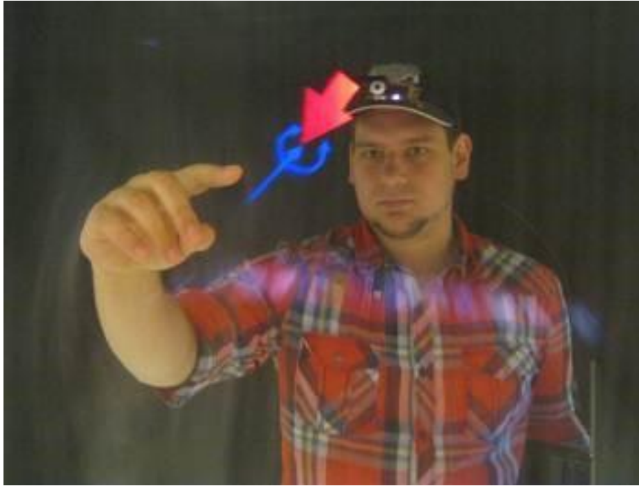
Figure 4. HMPP on a large fogscreen allows for multi-user content sharing without participants obstructing the projection.
