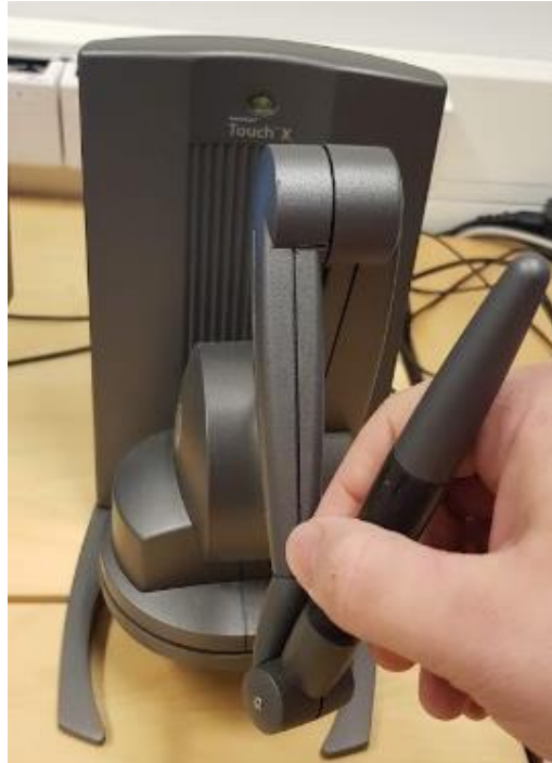
Figure 12. A 3D Systems Touch X haptic device.
