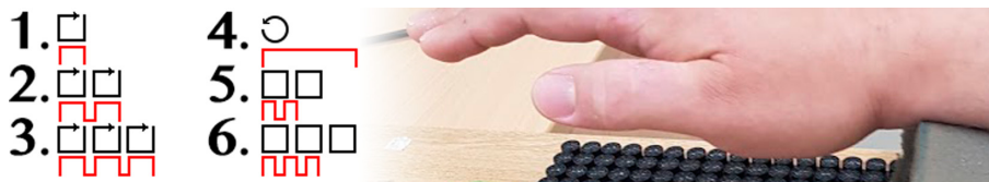
Fig. 1. Rendered shapes and repetitions. In stimuli 1 to 4, the focal point movement can be perceived, as shown by the arrow. Stimuli 5 and 6 use spatiotemporal modulation, making the entire shape concurrently perceivable.
