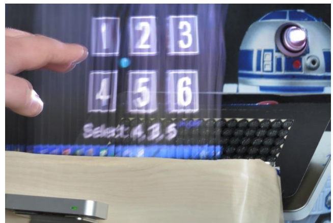
Fig. 2. A user is pressing keys on a particle screen with finger tracking and tactile feedback. From front left to back right: Leap Motion Controller, FogScreen, phased ultrasonic 16x8 array and projector (masked with an R2D2 printout).
