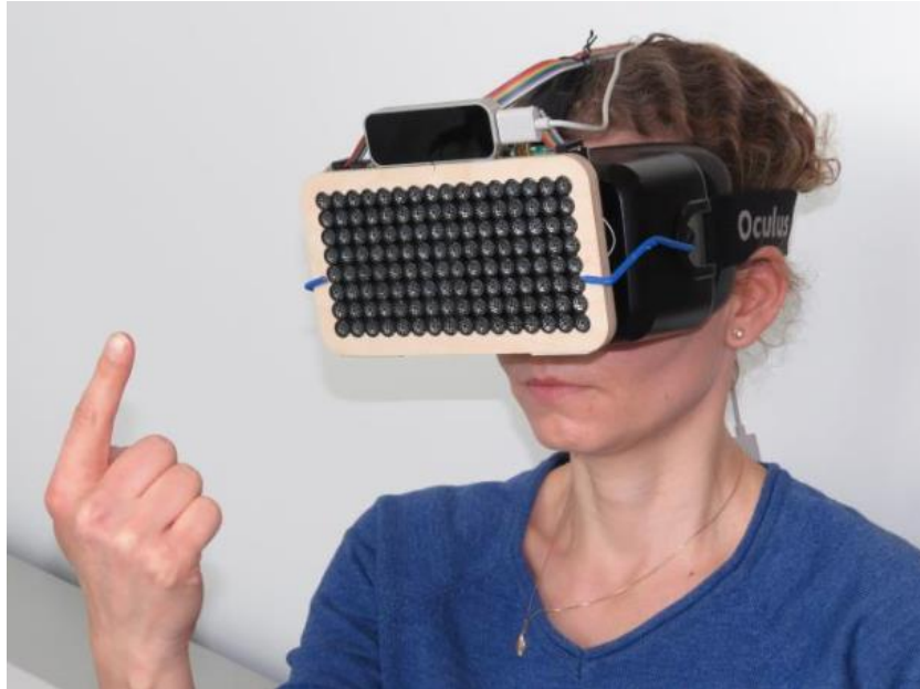
Figure 7. An ultrasonic mid-air haptics device attached to a head-mounted display always keeps the feedback oriented to facing direction. The hand tracking sensor on top of the matrix allows the focal point to be directed at the fingertip.
