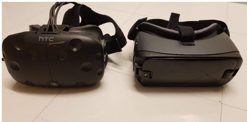
Figure 6. Head-mounted displays. On the left is an HTC Vive HMD; on the right is a Samsung Gear VR HMD.
