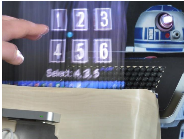
Figure 19. From front left to back right: Leap Motion controller, FogScreen, phased ultrasonic 16x8 array, and projector (masked with an R2D2 printout).
