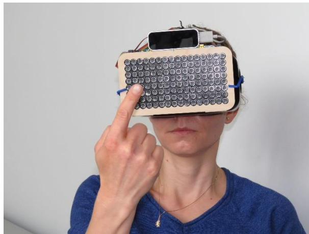
Figure 20. A modulated ultrasonic phased array integrated into a head-mounted display can provide tactile feedback in mid-air. A LeapMotion hand tracker is attached on top of the array.
