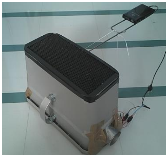
Figure 1: The hand-held fogscreen prototype construction.
