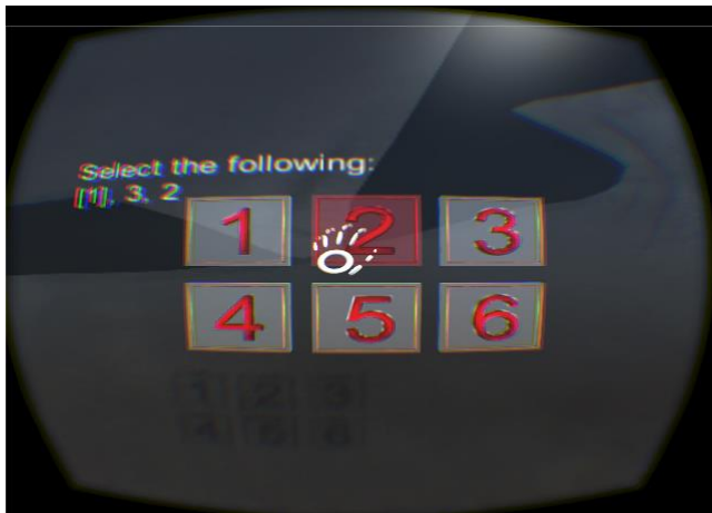
Figure 5: View of the virtual test environment with numerical keyboard. It shows also the skeletal representation of the user's hand touching a key and the key “2” in the red state that lasted for 0.2 seconds.
