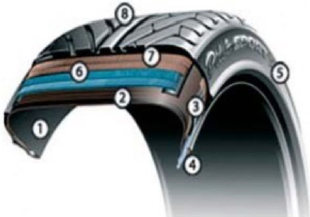
Figure 2. Key tire components (Tire Industry Project 2007)
