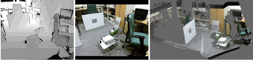
Figure 3.2 Sensor measurements from the Kinect v2 sensor. Left: Gray colored depth map encoding distance information from the surfaces of scene to the camera viewpoint. Foreground objects are colored darker and farther out are lighter. Middle: An RGB image aligned to the depth map. Some of the pixels are colored as black as they do not have corresponding pixel in the depth map. Right: resulting point cloud after inverse projection.
