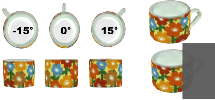
Figure 3.8 Example causes of pose ambiguity. Different poses of the mug cannot be recognized due to self-occlusion (left). Pose ambiguity introduced due to occlusion by another object (right).
