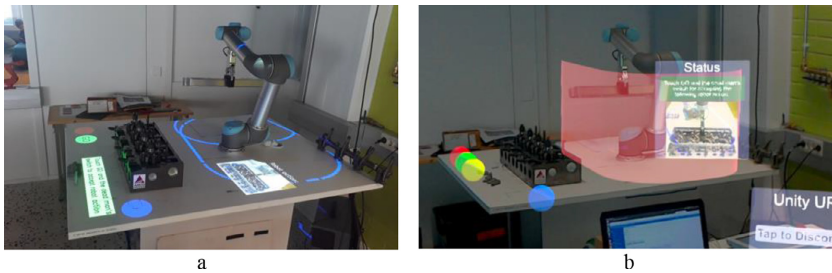
Fig. 1. The proposed interactive UIs for safe human-robot manufacturing: a) projector-mirror and b) wearable (AR) HoloLens. Video: https://youtu.be/WW0a-LEGLM .
