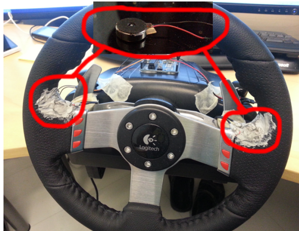
Figure 30: The wheel used in the experiment with attached actuators
