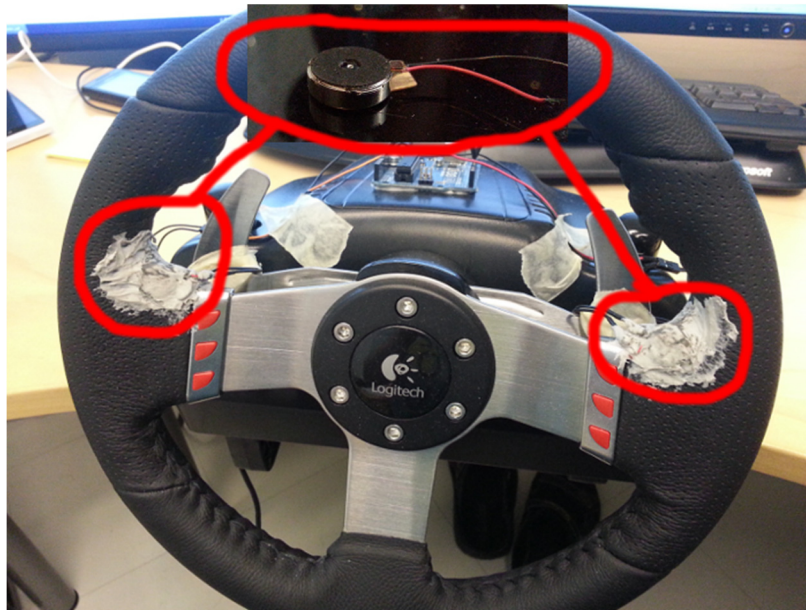
Fig. 1. The wheel setup including two actuators used for haptic feedback.
