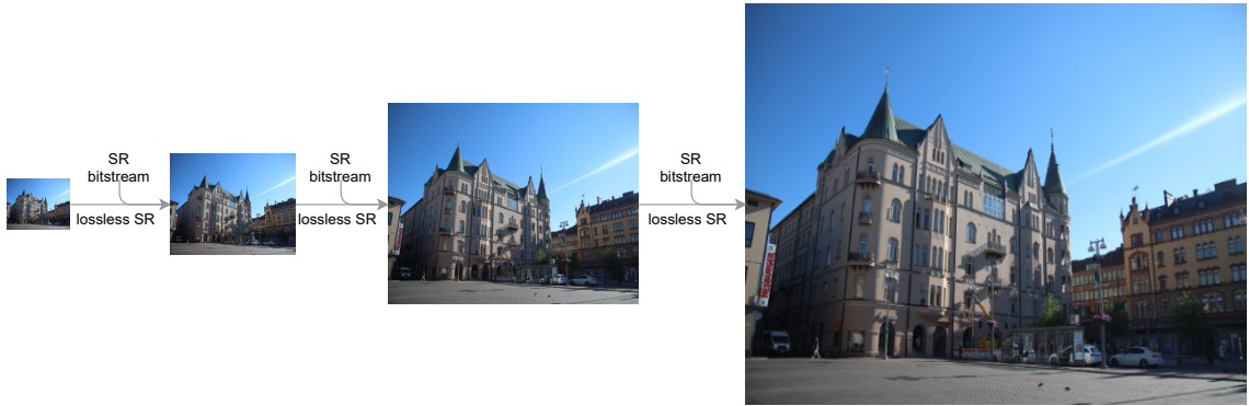
Figure 2.4 Image compression with super-resolution pipeline in [37]. Instead of compressing the full-size image, this scheme compresses the smallest-scale image and the lossless super-resolution bitstreams (SR bitstreams) of the subsequent scales.
