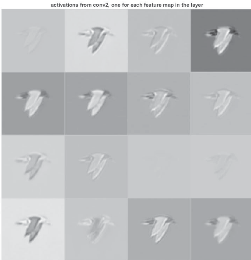
Fig. 6. Visualization of the feature extraction by the CNN model for the class LBBG. There are 16 feature maps in the figure extracted by the second convolution layer.
