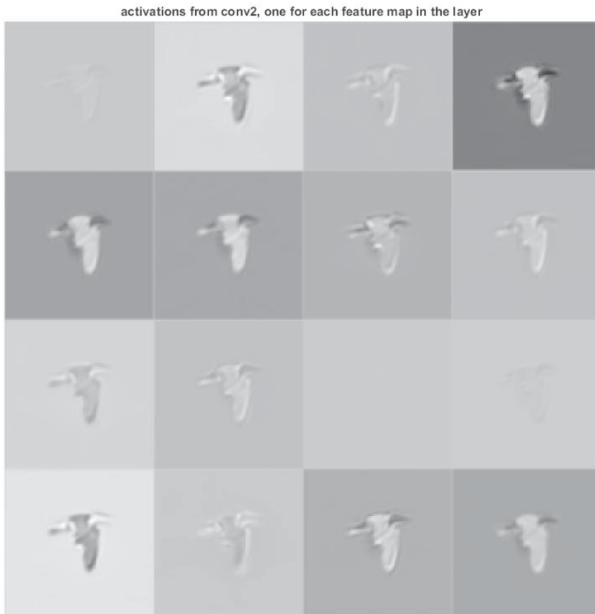
Fig. 7. Visualization of the feature extraction by the CNN model for the class GBBG. There are 16 feature maps in the figure extracted by the second convolution layer.
