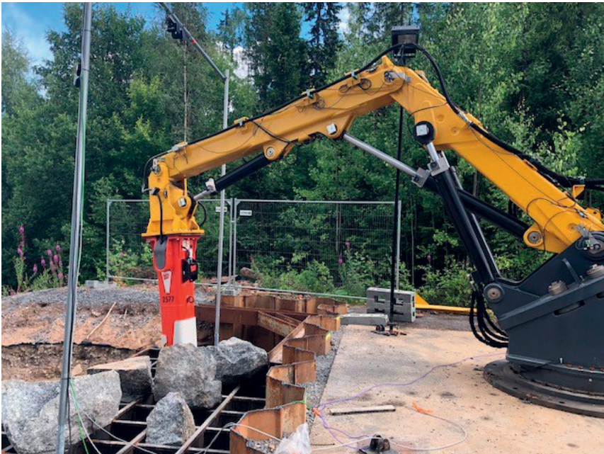
Figure 2.6 The scene of secondary breaking with guidance of a IFM O3M150 time-of-flight (TOF) camera.
