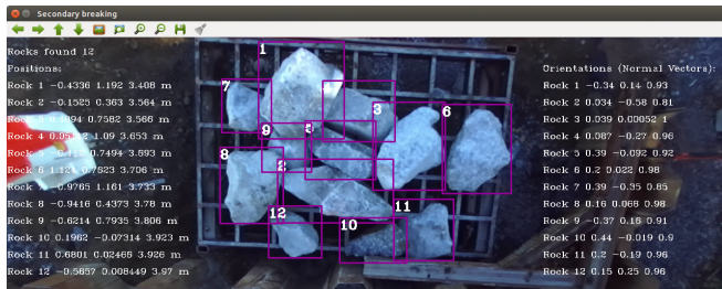
Fig. 6 Detection and localization of rocks at approx. 15Hz
