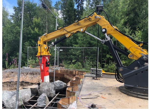
Figure 1: Secondary breaking with guidance of the ToF camera
