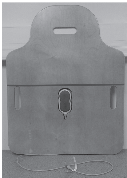
Fig. 1. Backboard with a compression force and deflection sensor (FDS) set under the patient's back so that the dark line is at the patient's axillary level. The dimensions of the backboard were 62 cm × 78 cm × 0.8 cm and weight was 2.8 kg, placed under the patient across the bed and reached up from head-to-hips.
