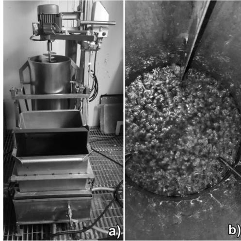
**Figure 6.1** (a) Laboratory scale foam forming equipment; (b) NFC-CNT dispersion, pulp, and water mixture before foaming [Publication III].
