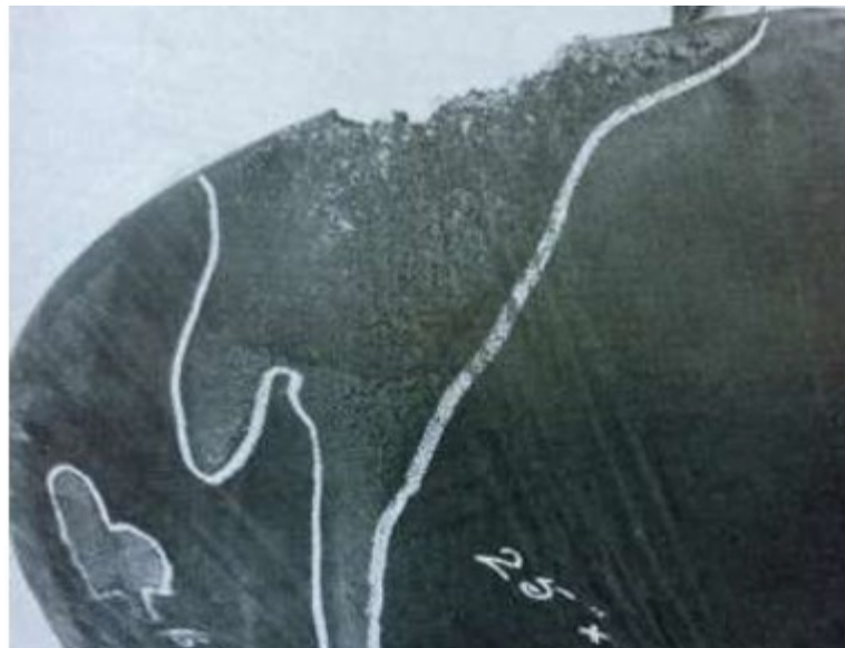
Figure 9. Cavitation damage on a propeller blade. (Stone Marine Propulsion Ltd, 2019)
