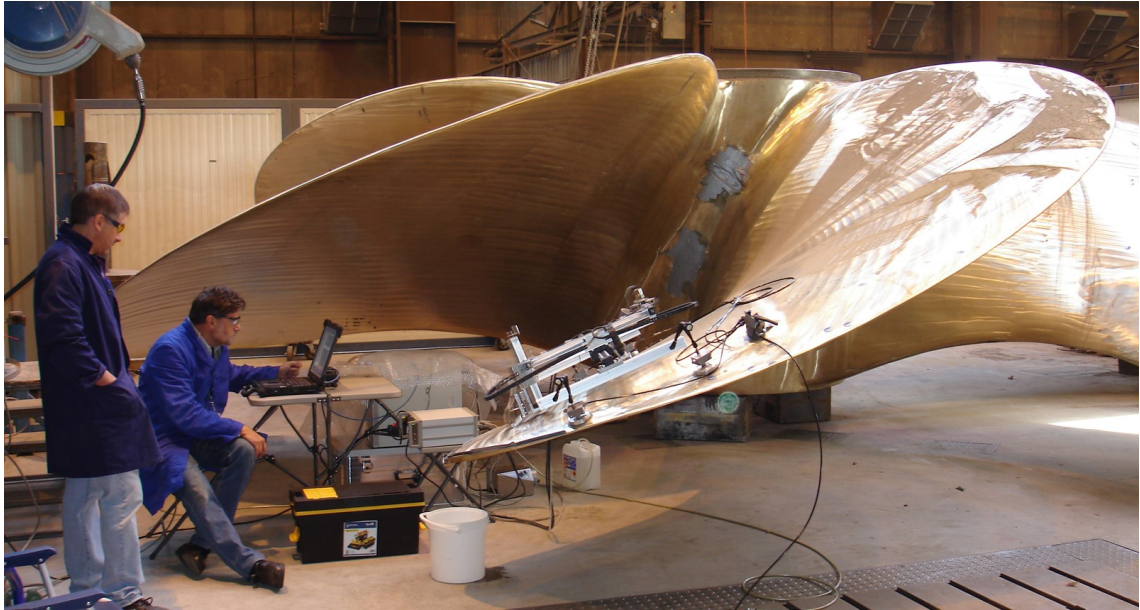
Figure 5. Ultrasonic testing of a propeller. (Fraunhofer-Gesellschaft, 2012)
