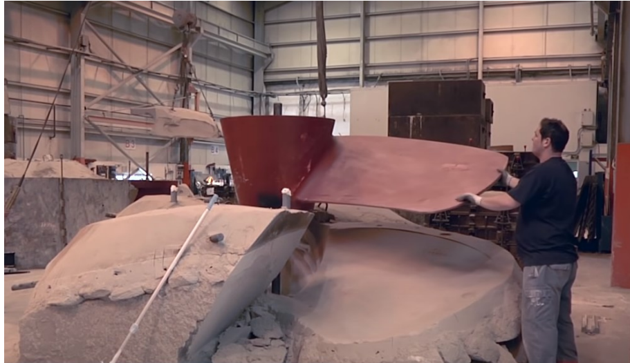
Figure 2. Pattern used for making casting mold. (Wärtsilä, 2016)
