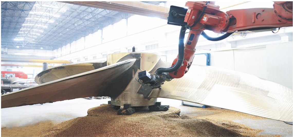
Figure 4. Propeller blade machining. (Yuanhang propellers manufacturing Co Ltd, 2020)
