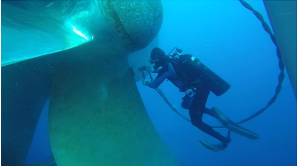
Figure 6. Diver polishing a propeller. (Odfjell, 2019)
