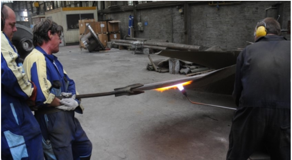
Figure 7. Hot straightening of propeller. (AEGIR-Marine, 2020)
